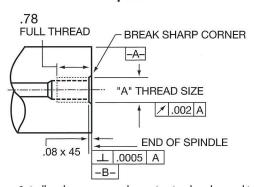
Note: Spindle tolerances must be maintained under working loads to assure proper operation.
